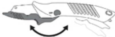
Protection Set Can Receive The Knife And Be Used For Assist In Stripping Sheathed Wire.
